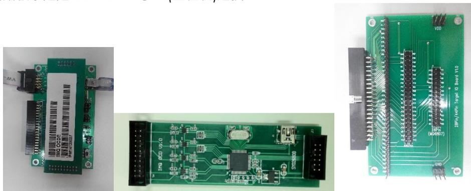
图 2.1 EV board 图 2.2 OCD board 图 2.3 Target board
